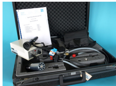
Bendoscope-Set for Power Plant Inspection (SF6 Switches)
