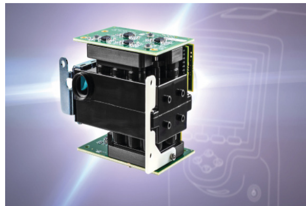
Optoelectronic module for a Molecular Diagnostics POCT device
