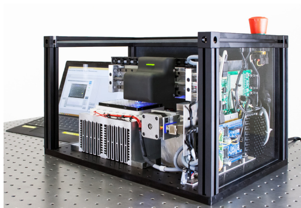
Breadboard test system with full functional integration of optics and thermal sample control for qPCR
