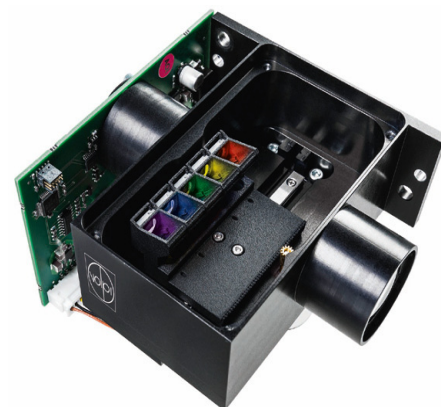
Illumination and detection solution applying spectral channel switching
